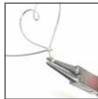
4. Trim the straight wire so that it is only about 1/2 inch long. Use the round nose pliers to make a small closed loop but still leave a little space above the loop.
